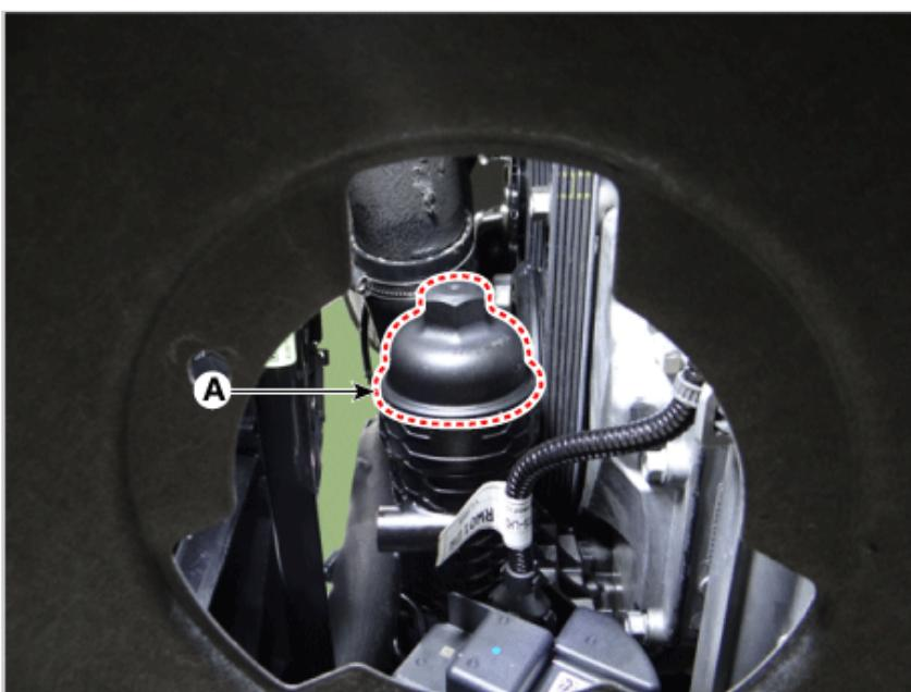
(3) Replace the O-ring (A) of oil filter cap with a new one.
