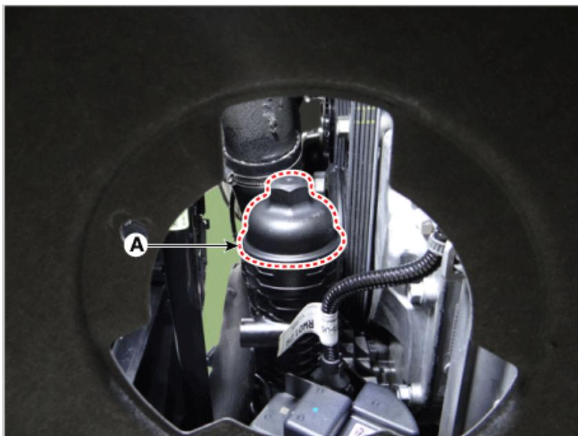
(3) Replace the O-ring (A) of oil filter cap with a new one.
