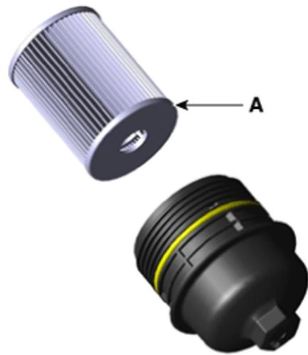
(5) Check and clean the oil filter installation surface.
