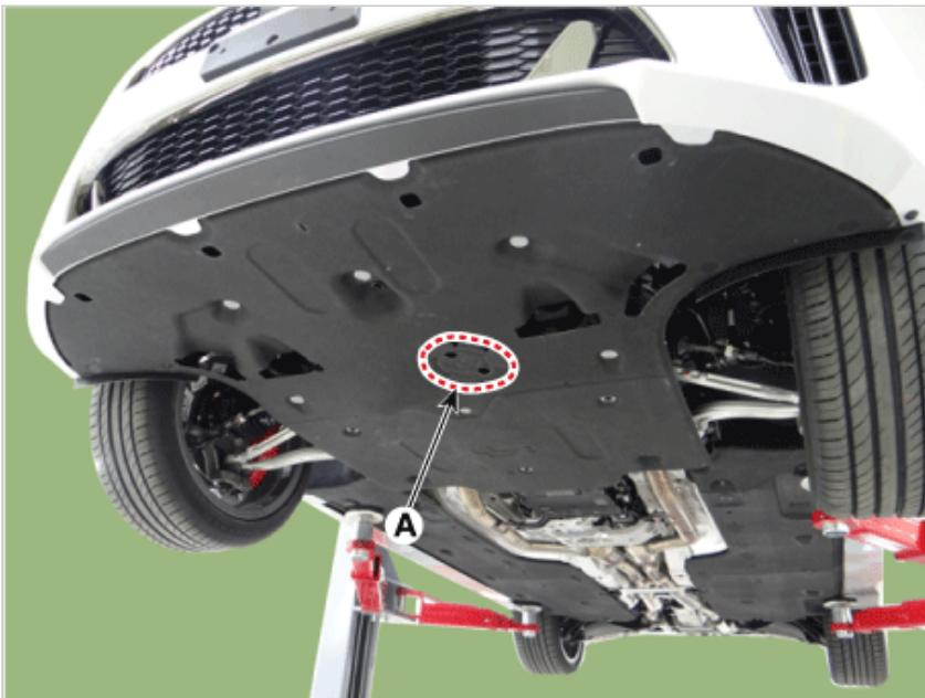
(2) Remove the oil filter cap (A).
